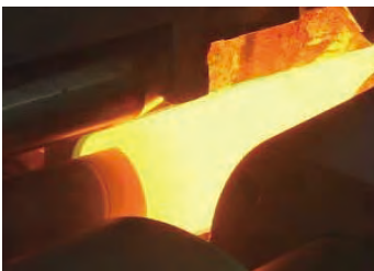
Seamless steel pipe piercing experiment (for OCTG/linepipe)
