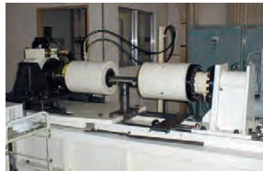
Large scale torsion fatigue testing machine
